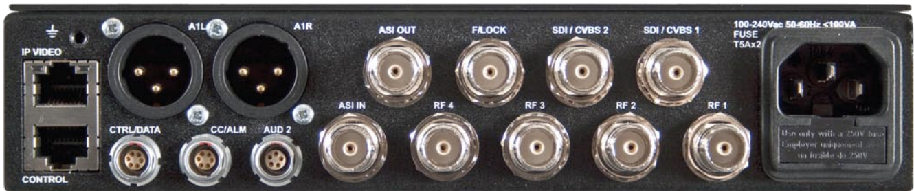
Lynx Diversity Receiver Connections
